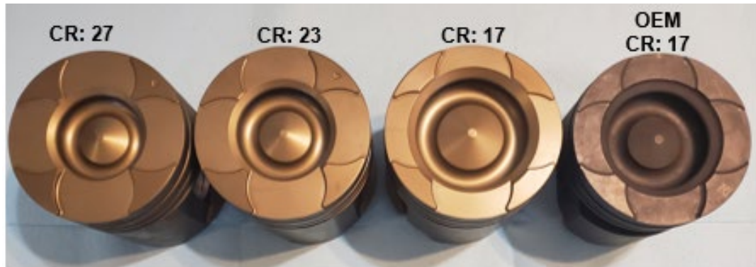
Figure 4.34: Aftermarket Piston to OEM Bowl Comparison (Manufactured)
